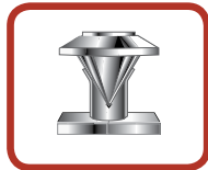
Flares rolled out above die bar.
