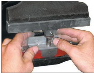
Bench vise used vertically as a press.
