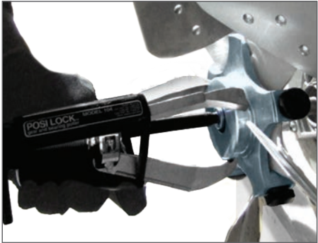
Makes cooling fan removal a one-person operation.
